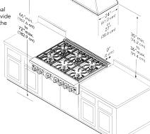
Important: This rangetop comes standard with an Island Trim. There must be a minimum of 6" (15.2 cm) clearance from rear of rangetop to a combustible wall. Clearances from non-combustible materials are not part of the ANSI Z21.1 scope and are not certified by CSA. Clearances to non-combustible materials must be approved by the authority having jurisdiction.
