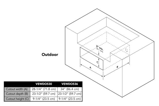
Note: For Outdoor Models, seal around drawer opening with silicon caulk that is provided.
