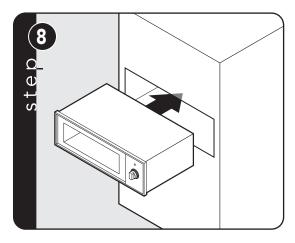
Slide cavity assembly into the cabinet opening.
