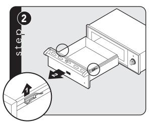
Slide finger along right and left side until you reach the black hand latches (located at the front of the rails). Pull up on both the right and left latches and pull out drawer pan support.
