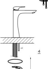
5. CONNECT THE FEMALE END OF FLEXIBLE HOSES TO THE COLD AND HOT WATER SUPPLY.
