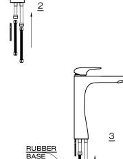
3. PLACE THE RUBBER BASE IN TO THE SLOT AT THE BOTTOM OF THE FAUCET
