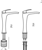
4. PLACE NEW FAUCET IN THE POSITION ON THE SINK. PLACE BRASS RING BETWEEN BOTTOM OF THE FAUCET AND SINK SURFACE. FROM UNDER THE SINK, PUT RUBBER WASHER AND THREAD NUT ONTO THE PIN. TIGHTEN NUT.
