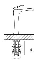
5. CONNECT FLEXIBLE HOSES TO THE COLD AND HOT WATER SUPPLY.
