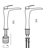
4. PLACE NEW FAUCET IN THE POSITION ON THE SINK. PLACE BRASS RING BETWEEN BOTTOM OF THE FAUCET AND SINK SURFACE. FROM UNDER THE SINK, PUT RUBBER WASHER AND THREAD NUT ONTO THE PIN. TIGHTEN NUT.
