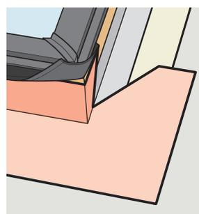
**ENGLISH:** To ensure waterproofing, skylight frames should be completely wrapped in VELUX adhesive skylight underlayment supplied with the flashing. This underlayment must be applied before installing the flashing.
