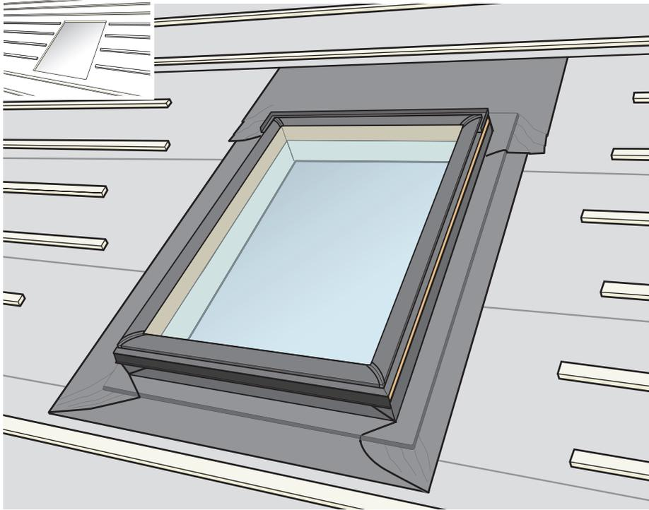
**ENGLISH: Installing VELUX adhesive skylight underlayment on roof with battens:**
