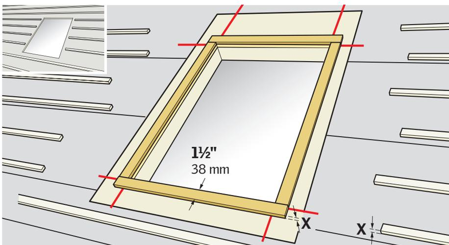
**ENGLISH: Roof with battens:** Place 1½" (38 mm) wide battens around rough opening. Batten thickness around rough opening should be equal to thickness of battens used for roofing material.
