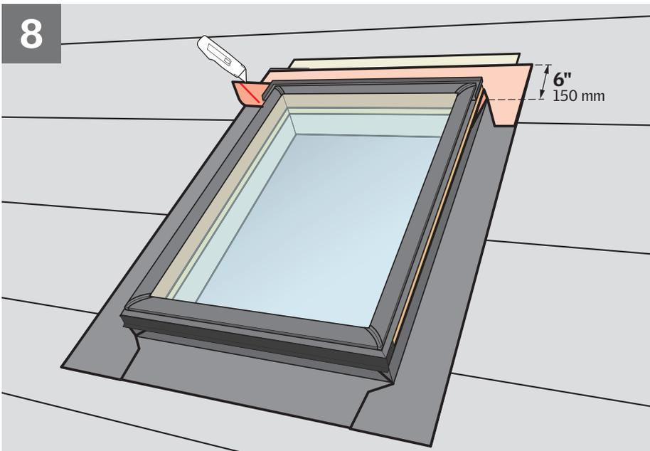
**ENGLISH:** Wrap the top frame and corners of the skylight with VELUX adhesive skylight underlayment and create proper water-shedding lap.
