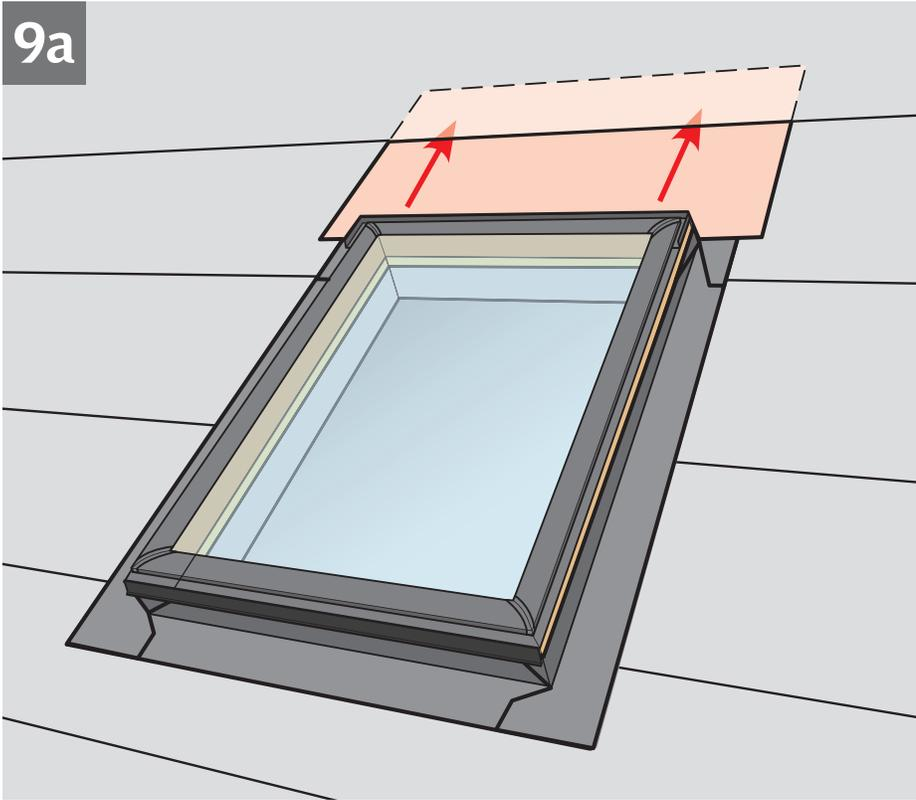
**ENGLISH:** To allow for proper drainage, interweave roofing underlayment as shown in **9a** for new construction applications. For retrofit applications, interweave roofing underlayment as shown in **9b**.
