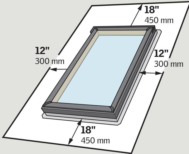
**ENGLISH:** Maintain illustrated clearances between skylight frame and critical areas such as valleys, ridges, slope changes and roof-to-wall intersections.
