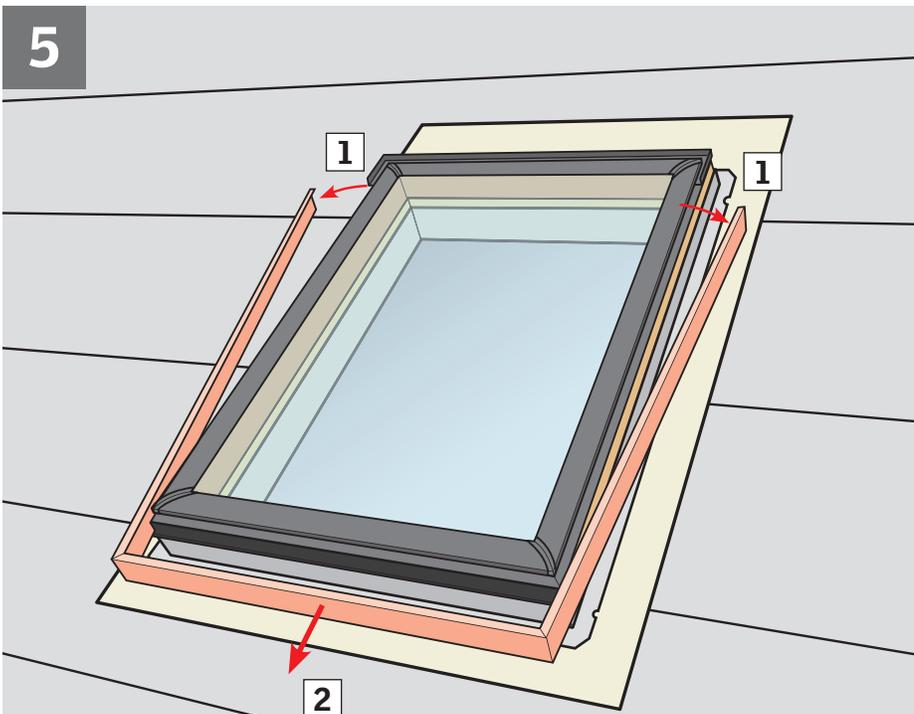
**ENGLISH:** To properly install VELUX adhesive skylight underlayment, remove cladding as shown.
