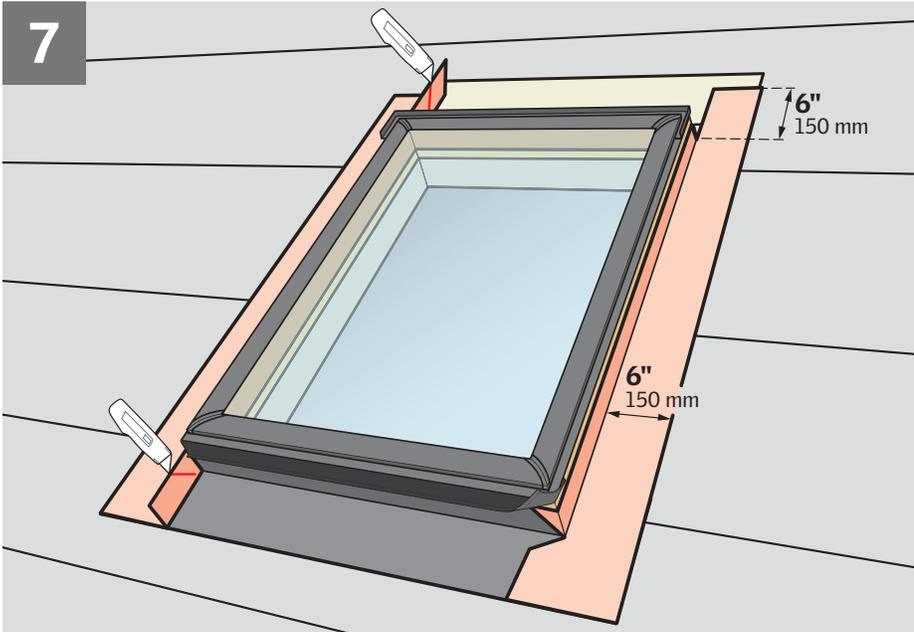
**ENGLISH:** Wrap the side frames and corners of the skylight with VELUX adhesive skylight underlayment and create water-shedding laps over roofing underlayment.
