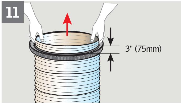
**ENGLISH:** Pull 3" (75 mm) of the flexible tunnel through the pivot ring.
