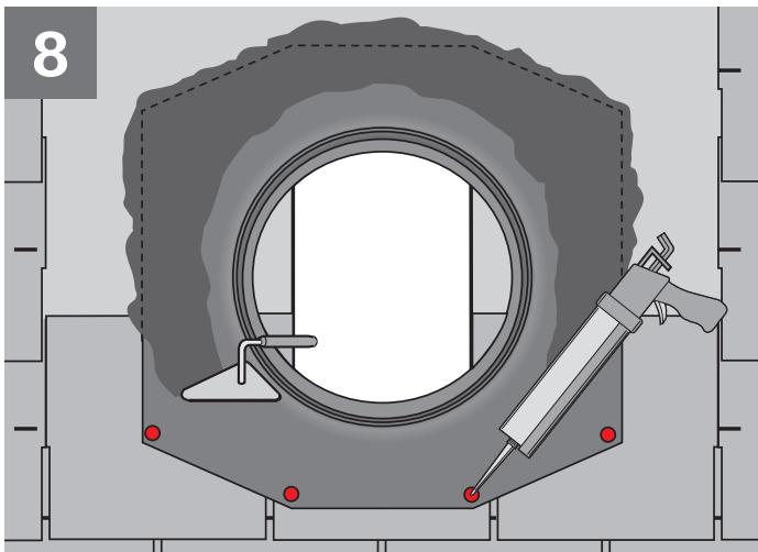
**ENGLISH:** Apply sealant as shown, and seal all fasteners.
