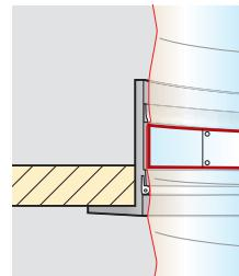
**ENGLISH:** Move the locking snap ring to final position as shown – 3/8" (10 mm) above the position for the diffuser.
