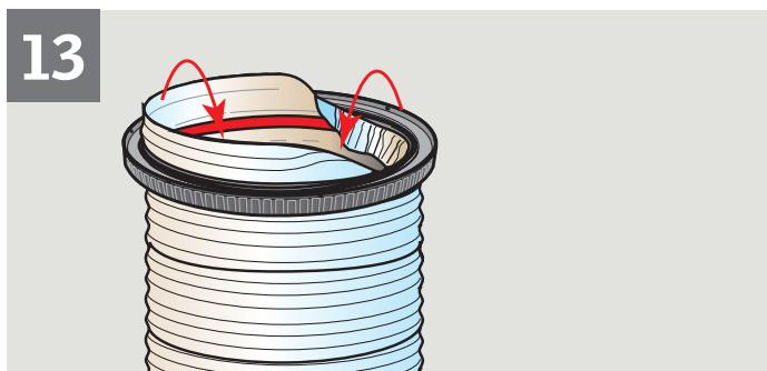
**ENGLISH:** Fold end of the tunnel over the locking snap ring, and secure the loose edge of tunnel with tape provided.
