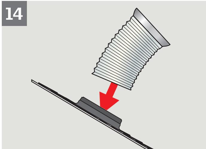
**ENGLISH:** Insert tunnel assembly into the flashing.
