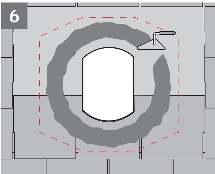
**ENGLISH:** Remove the roofing material around the upper half of the rough opening as indicated and apply mastic around rough opening as shown.
