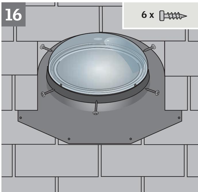
**ENGLISH:** Align holes; install and secure the dome with the  $\frac{3}{8}$ " (19 mm) screws provided. Do not overtighten the screws.
