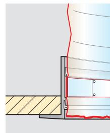
**ENGLISH:** Cut off excess tunnel flush with the ceiling ring as shown.
