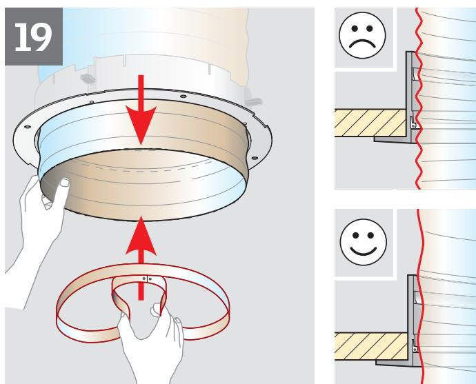
**ENGLISH:** Fold and insert the  $\frac{3}{4}$ " (19 mm) locking snap ring to lock the flexible tunnel in place. Pull the flexible tunnel tight.
