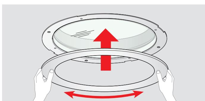
**ENGLISH:** Install the trim ring by aligning notches, and rotate to secure.
