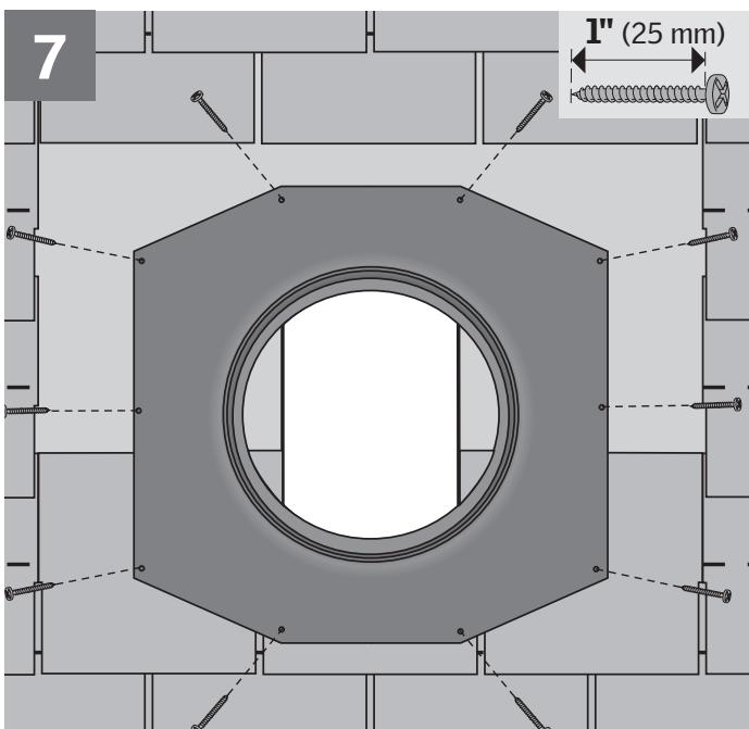
**ENGLISH:** Center the flashing over the rough opening, and secure the flange with ten of the provided 1" (25 mm) screws in all the pre-punched holes along the edges.
