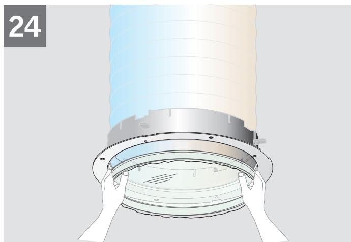
**ENGLISH:** Install the diffuser with the frosted side facing down.
