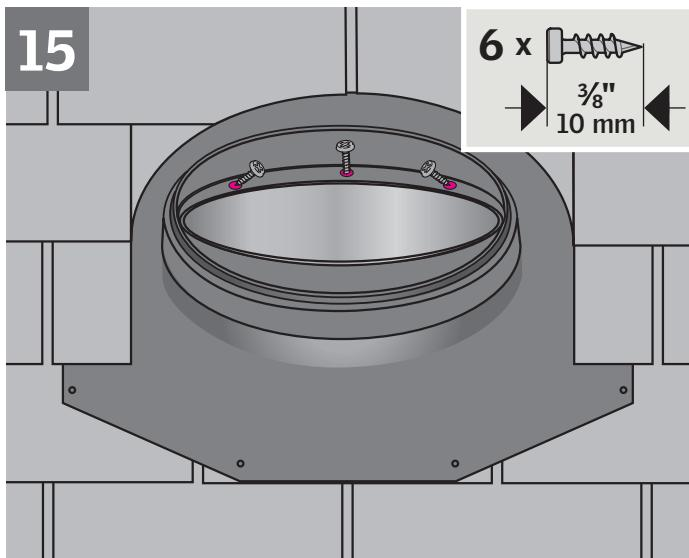
**ENGLISH:** Seat the pivot ring with the tunnel assembly into the flashing. Secure the pivot ring with screws if needed.
