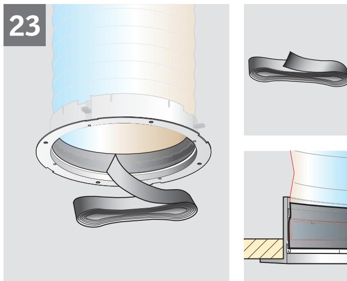
**ENGLISH:** Secure the loose edge of tunnel with tape provided.
