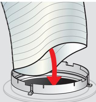
**ENGLISH:** Pull the flexible tunnel section down through the ceiling ring.
