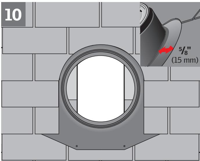
**ENGLISH:** Reinstall roofing material over the flange. Leave a  $5/8"$  (15 mm) channel for water to run off. Optional turret extensions ZTA are available where domes need to be elevated by  $6\frac{1}{2}"$  (165 mm) or  $9"$  (230 mm).
