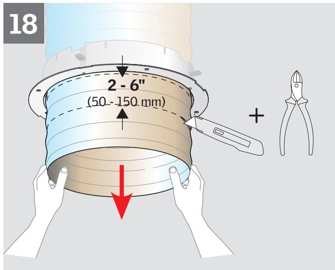
**ENGLISH:** Pull the flexible tunnel section tight through the ceiling ring, and cut flexible tunnel to length as shown.
