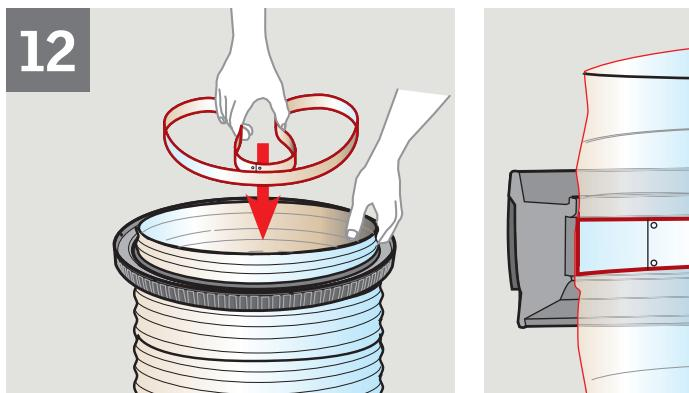
**ENGLISH:** Fold and insert the  $\frac{3}{4}$ " (19 mm) locking snap ring to lock the flexible tunnel in place. Move the locking snap ring to final position as shown.
