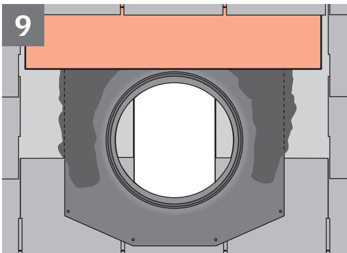
**ENGLISH:** Overlap the top of the flange with underlayment to allow for proper drainage.
