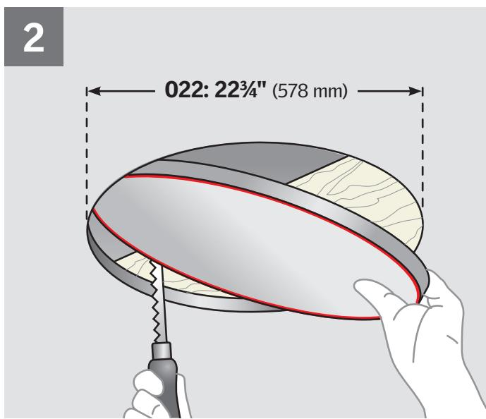
**ENGLISH:** Carefully remove the other parts from the ceiling ring. Rotate trim ring to disengage.
