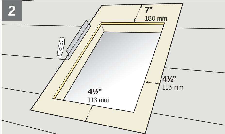
**ENGLISH:** Remove existing roofing underlayment around the rough opening as shown.
