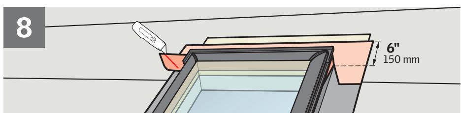
**ENGLISH:** Wrap the top frame and corners of the skylight with VELUX adhesive skylight underlayment and create proper water-shedding lap.
