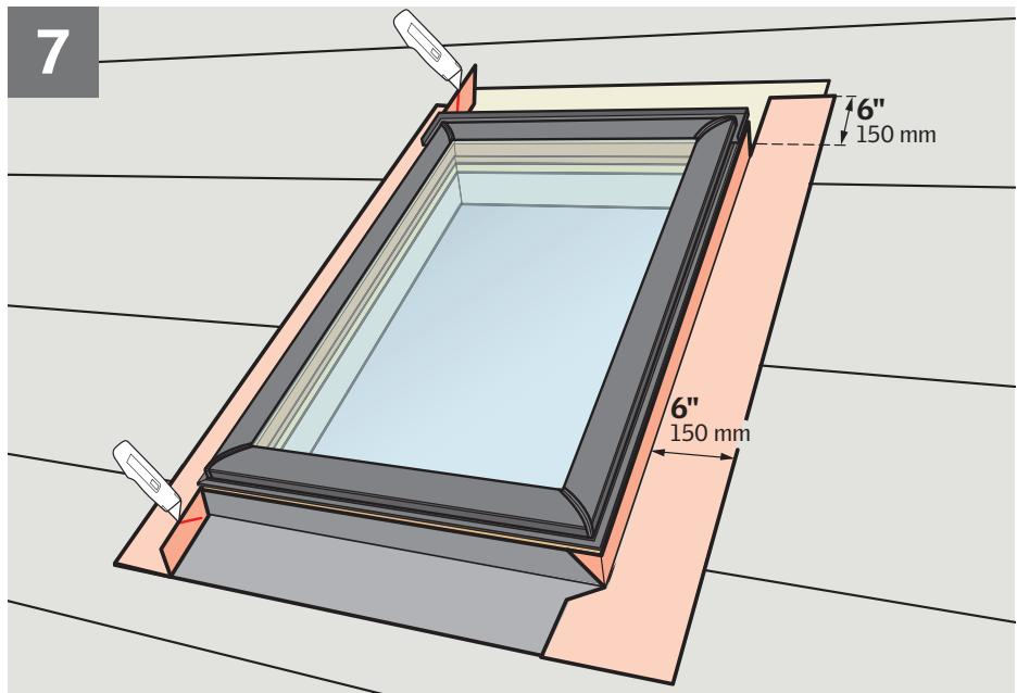
**ENGLISH:** Wrap the side frames and corners of the skylight with VELUX adhesive skylight underlayment and create water-shedding laps over roofing underlayment.
