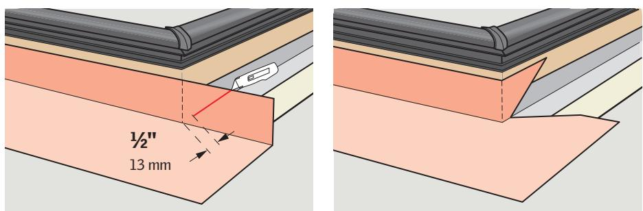
**ENGLISH:** To ensure waterproofing, skylight frames should be completely wrapped in VELUX adhesive skylight underlayment supplied with the flashing. This underlayment must be applied before installing the flashing.
