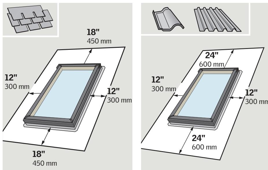
**ENGLISH:** Maintain illustrated clearances between skylight frame and critical areas such as valleys, ridges, slope changes and roof-to-wall-intersections.
