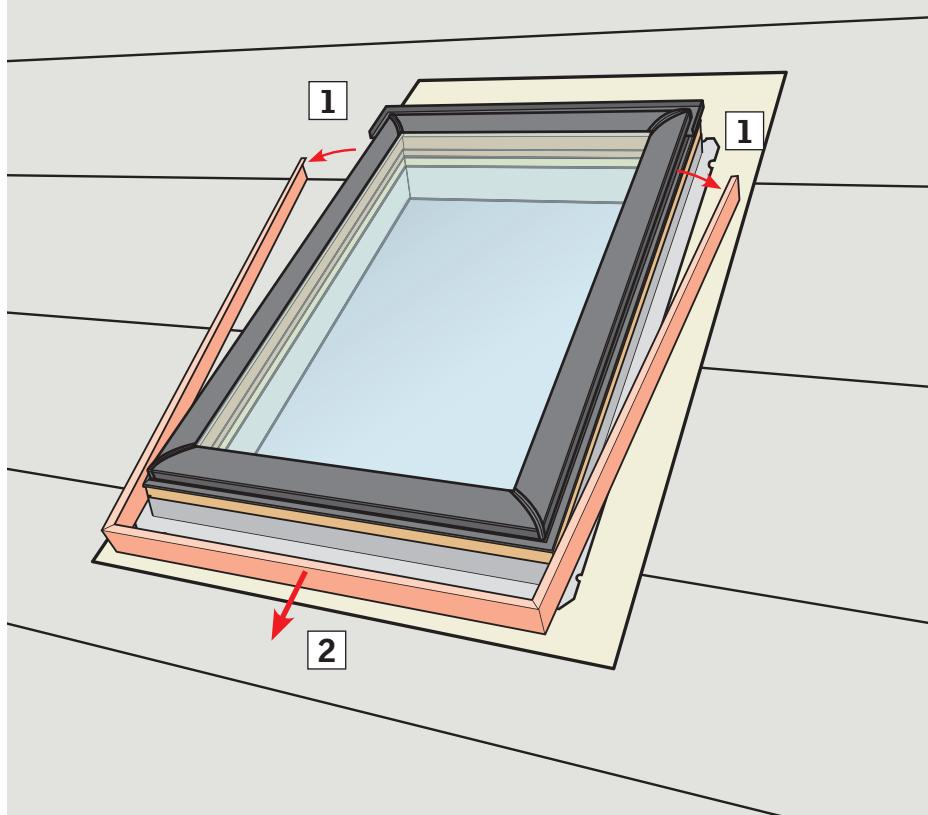
**ENGLISH:** To properly install VELUX adhesive skylight underlayment, remove cladding as shown.
