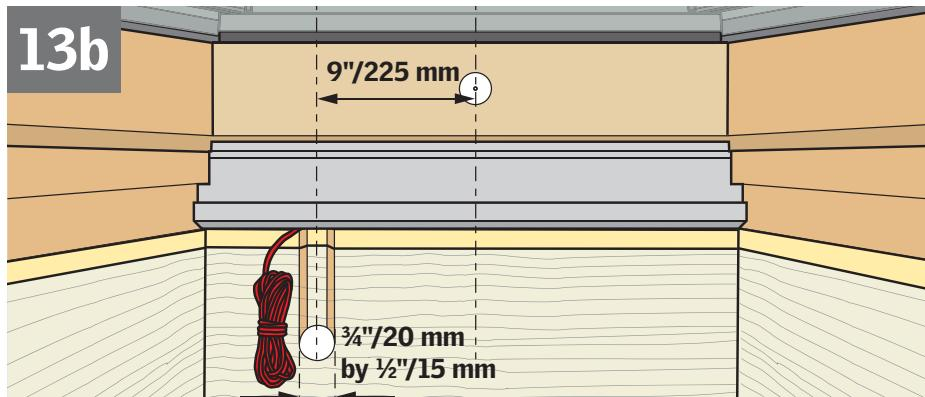
**ENGLISH:** Prepare the framing for electrical wiring. All wiring shall be done with factory attached power cable. Wiring of power cable shall be done in accordance with the latest edition of the National Electrical Code (NFPA 70) and all local codes and ordinances.
