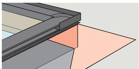
**ENGLISH:** To allow for proper drainage, interweave VELUX adhesive skylight underlayment as shown in 9a for new construction applications. For retrofit applications, interweave VELUX adhesive skylight underlayment as shown in 9b.
