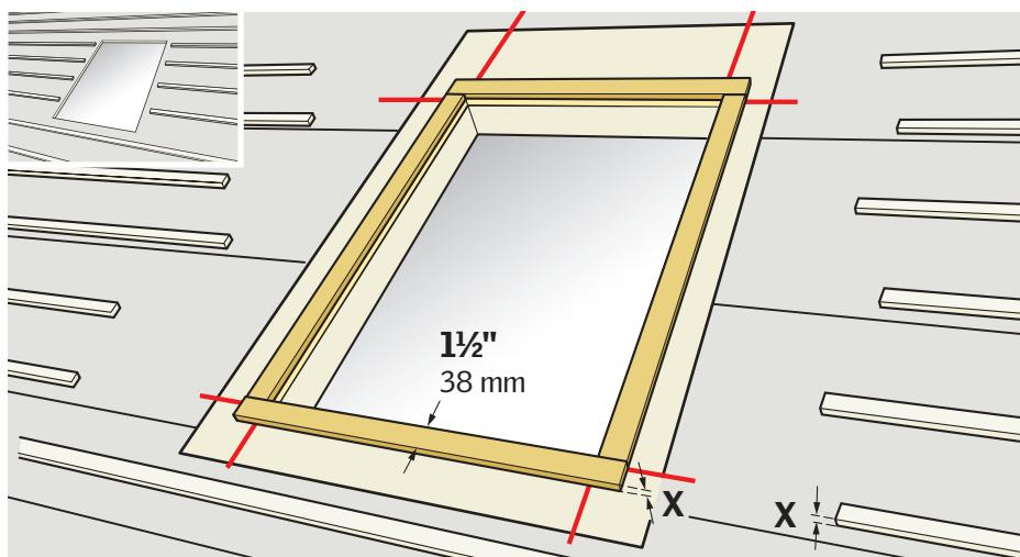
**ENGLISH:** **Roof with battens:** Place 1 1/2" (38 mm) wide battens around rough opening. Batten thickness around rough opening should be equal to thickness of battens used for roofing material.
