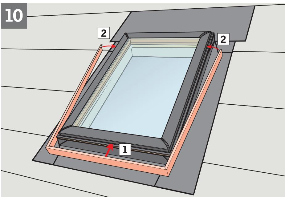
**ENGLISH:** You are now ready to install the flashing. If the flashing is not to be installed immediately, reinstall cladding.
