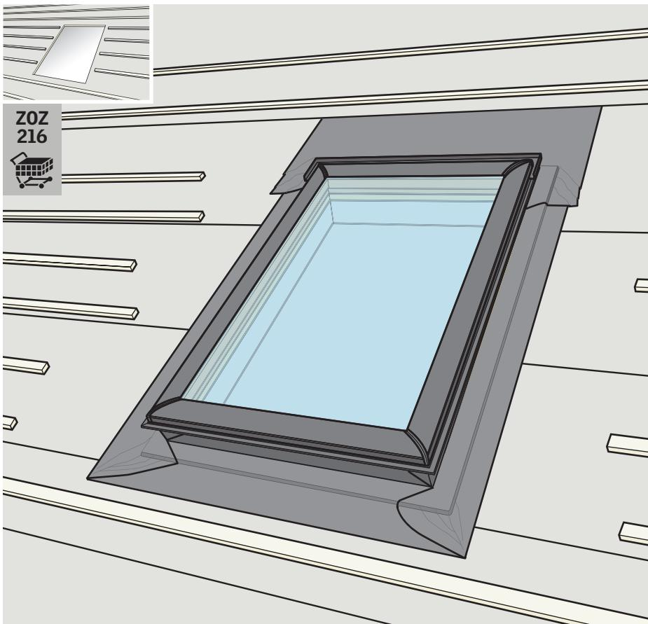
**ENGLISH:** Installing VELUX adhesive skylight underlayment on roof with battens:
