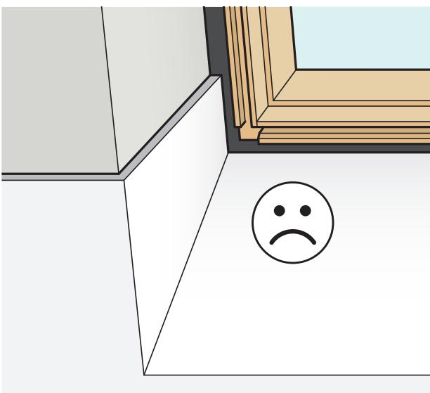
**ENGLISH:** If the drywall is not installed tight into the lining groove, add on-site insulation and trim for finished appearance and to prevent conditions that may contribute to condensation.
