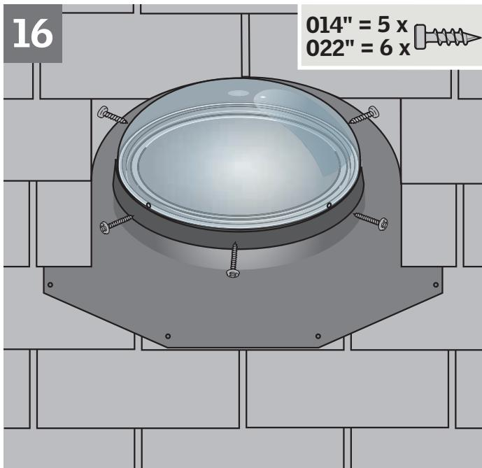
**ENGLISH:** Align holes; install and secure the dome with the  $\frac{3}{4}$ " (19 mm) screws provided. Do not overtighten the screws.
