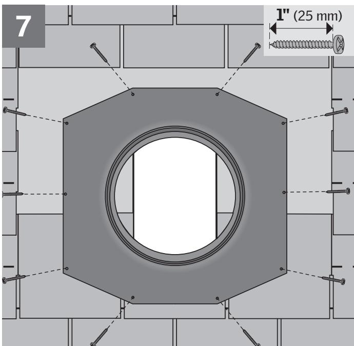
**ENGLISH:** Center the flashing over the rough opening and secure the flange with ten of the provided 1" (25 mm) screws in all the pre-punched holes along the edges.
