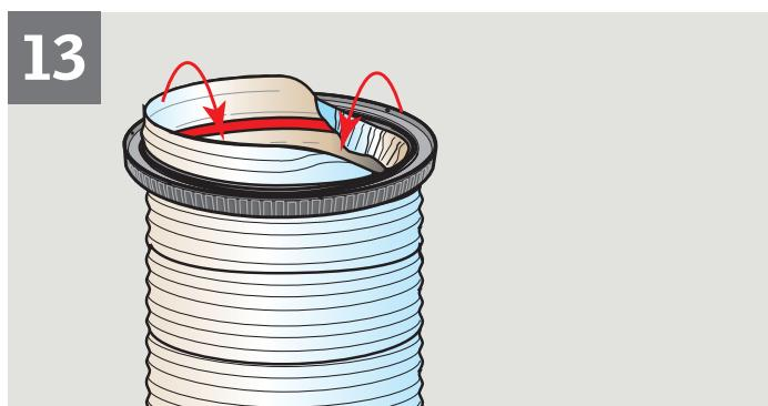
**ENGLISH:** Fold end of the tunnel over the locking snap ring and secure the loose edge of tunnel with tape provided.
