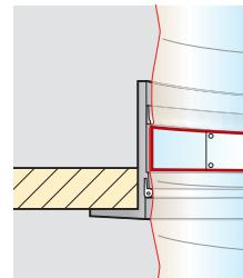
**ENGLISH:** Move the locking snap ring to final position as shown –  $\frac{3}{8}$ " (10 mm) above the position for the diffuser.
