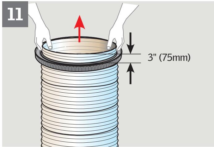
**ENGLISH:** Pull 3" (75 mm) of the flexible tunnel through the pivot ring.
