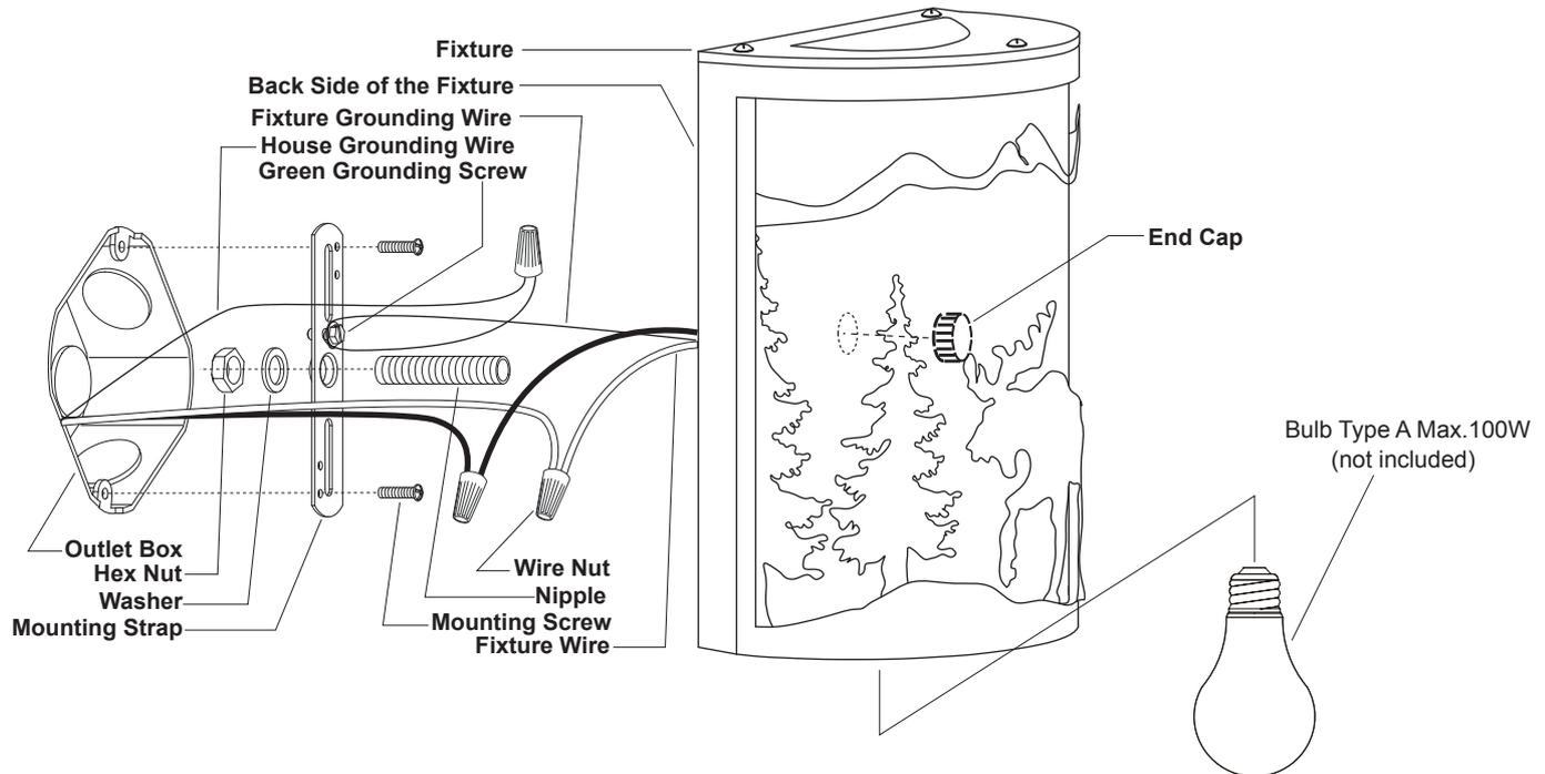
1. Attach the nipple to the mounting strap, then secure it with a washer and hex nut.
