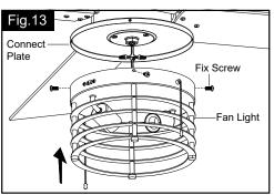
Connect the white (neutral) wire from the fan light to white (neutral) wire from fan motor assembly with a wire connector; connect the blue (hot) wire from fan light to Black (hot) wire from fan motor assembly with a wire connector. Carefully put the wires into the connect plate, then attach the fan light onto the connect plate with the four previous fix screws which was removed.
