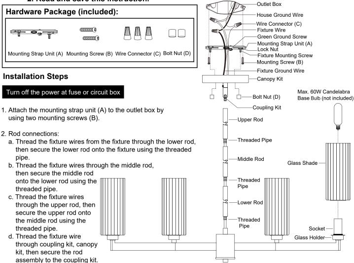
Note: Length adjustable from 10-3/4" to 55". Use fewer rods if shorter length is desired.
