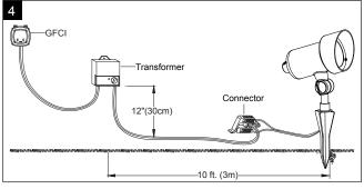
4. Attach the fixture to the power cable with the connector. To insure uniform brightness the first fixture should be a minimum of 10 feet (3 meters) from the transformer (not included). (Fig.4)
