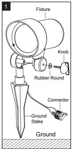
Align the power cable with the contact pins inside the connector and close the connector (Fig.3), making sure the contact pins pierce the power cable.
