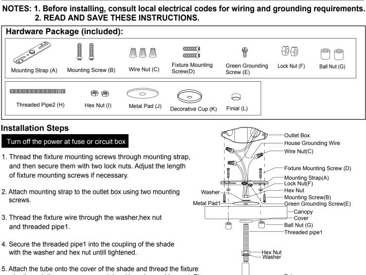
i. Attach the tube onto the cover of the shade and thread the fixture wire through the cover,canopy,metal pad1,washer and hex nut. Place the cover and canopy onto the tube through the threaded pipe1, then tighten them with the metal pad,
