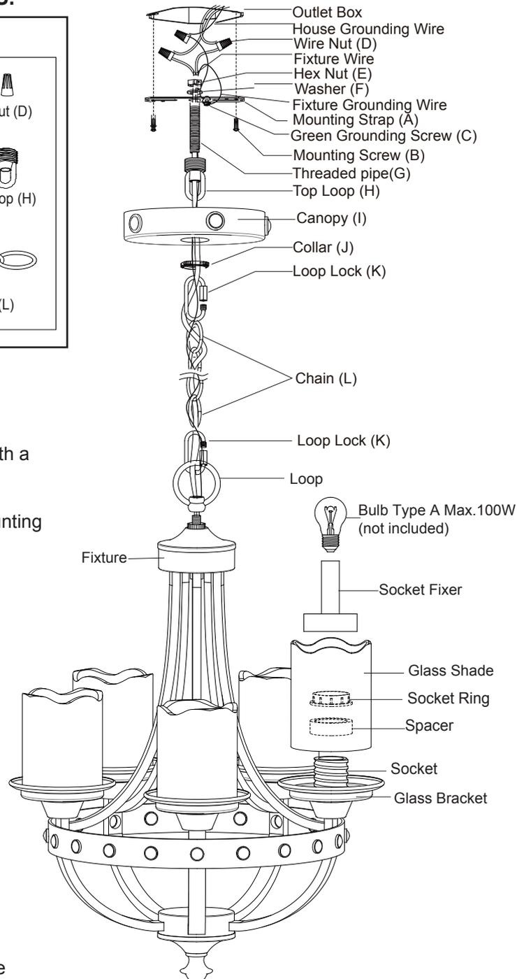
10. Attach the canopy to the mounting strap: insert the top loop through hole, then secure by tightening collar.
