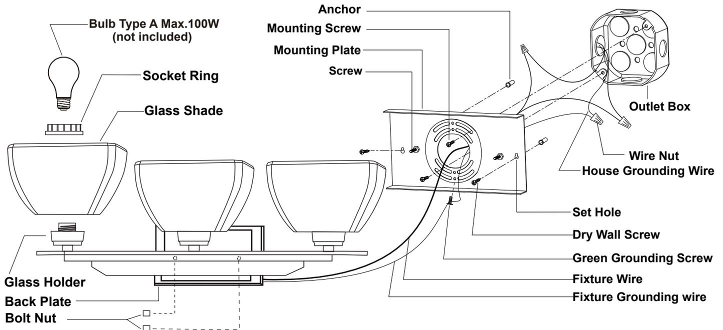
1. Unscrew the bolt nuts from the back plate, and then remove the mounting plate.
