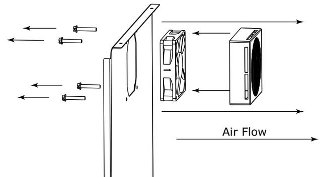
14. Remove and replace fan. Take special care to properly route fan wire.
