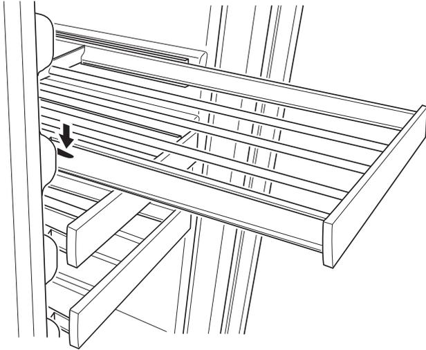
3. Press the left rack release lever down. At the same time, lift the matching right rack release lever up. Pull the rack out until it is free of the tracks and the cabinet.
