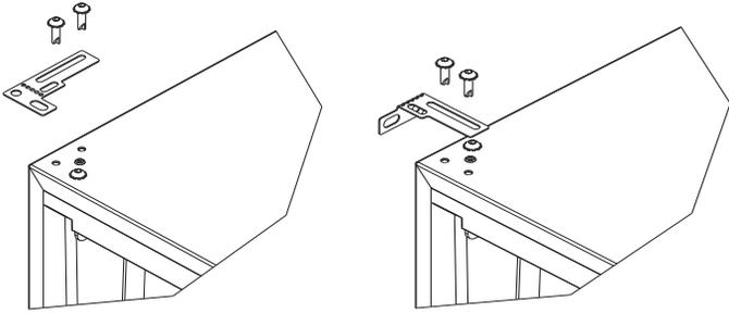
3. Place bracket over holes and attach to unit with two screws removed in step 2 using a T-25 Torx driver. Tighten screws fully.
