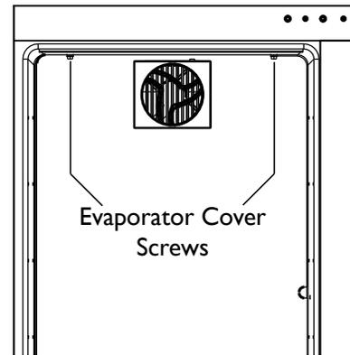
11. Grasp evaporator cover, pull forward and up as bottom of cover is installed behind the front edge of the drain trough.
