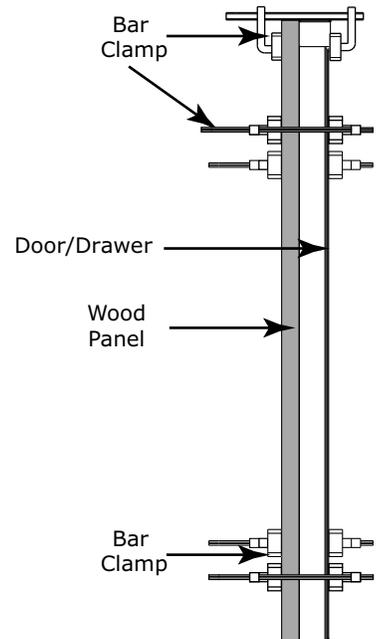
10. Using a 7/64" (3 mm) drill bit, drill 6 pilot holes into the wood panel 1/2" (12 mm) deep using the holes in the door/drawer frame as a guide.
