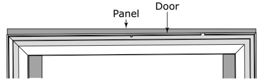
9. Secure integrated panel to door/drawer using clamps. A robust tape may also be used. U-Line recommends the use of bar clamps to secure the panel to the door/drawer. If using tape, be certain the tape will not damage panel finish upon removal.
