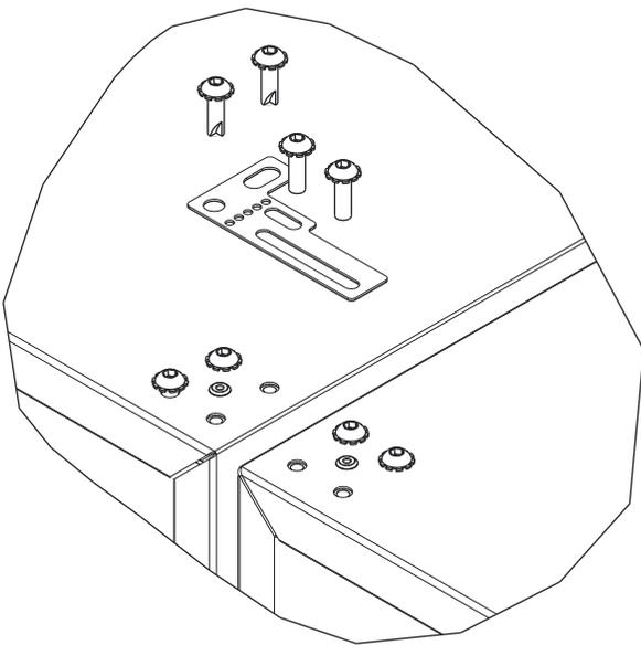
3. Place bracket over holes and attach to unit with two screws removed in step 2 using a T-25 Torx driver. Tighten screws fully.
