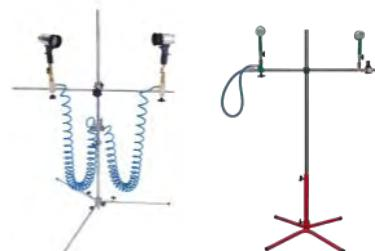
The higher the air pressure supply to air amplifier stands used with waterborne paint increases the amount of air volume they consume.
