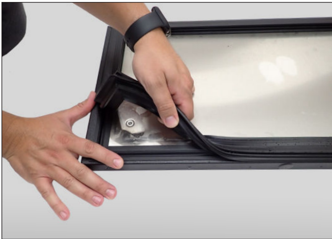
FIG. 3. Pull the gasket from the drawer.
