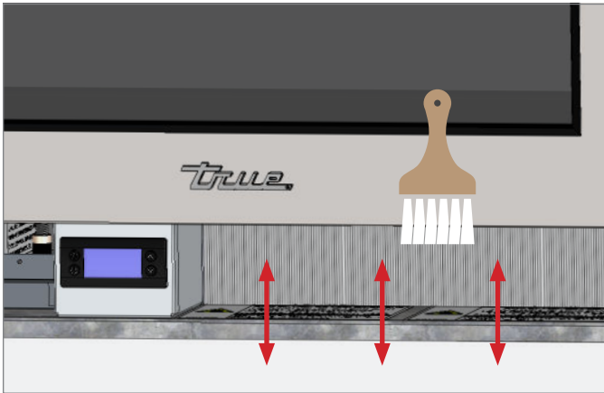
FIG. 2. Never brush across the coil fins.
