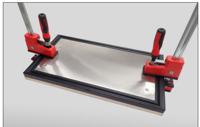
FIG. 5. Be sure the edges are aligned before clamping the drawer front assembly.
