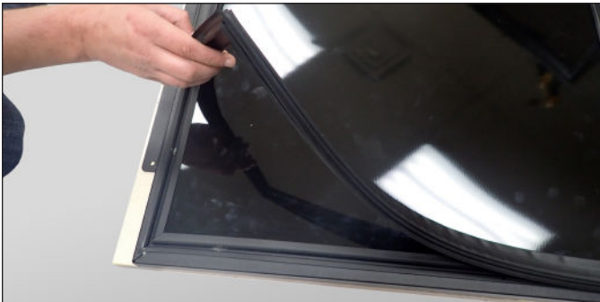
FIG. 3. Pull the gasket from the door.
