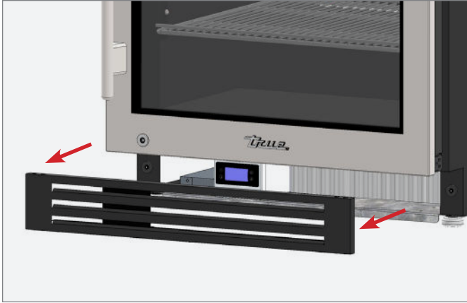
FIG. 1. Pull the kickplate off the magnets.
