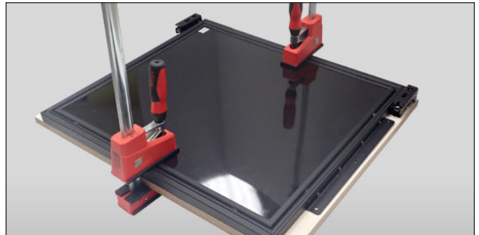
FIG. 4. Be sure the edges are aligned before clamping the door assembly.
