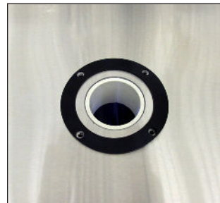
FIG. 1. Position the rubber gasket around the draft tower hole.
