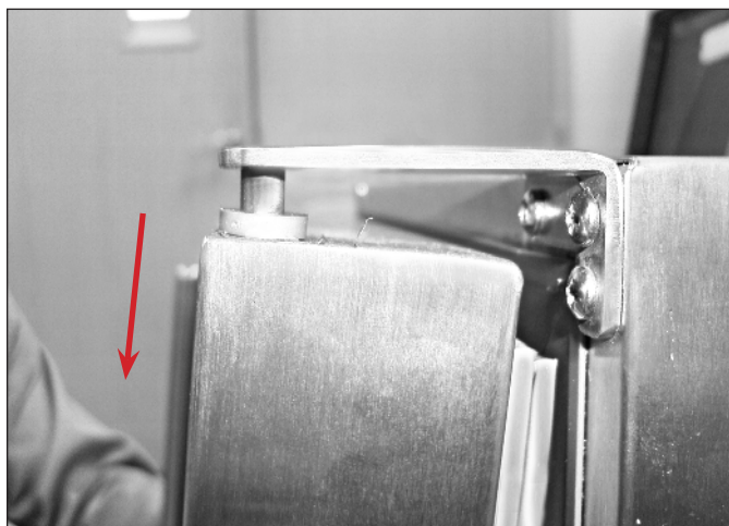
FIG. 3. Lower the door off the top hinge.
