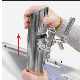
FIG. 5. Lift the top off the draft standard.
