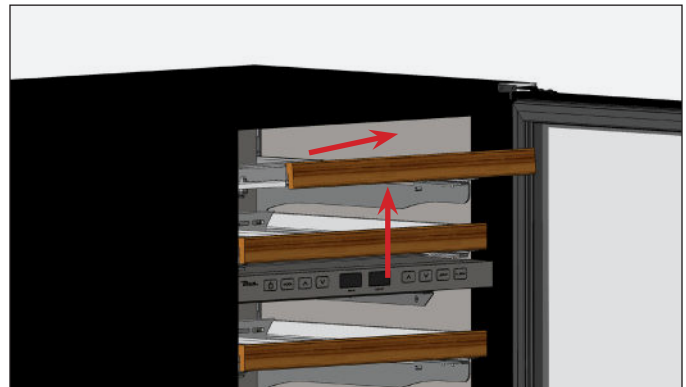
FIG. 1. Lift and pull the wine rack forward.
