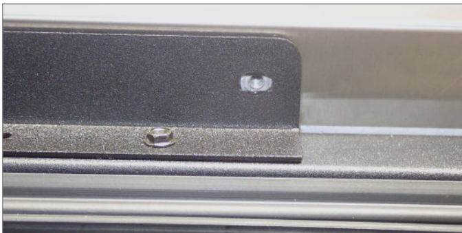
FIG. 3. Bracket screw holes are slotted for easy adjustment. Screw removed for illustration.
