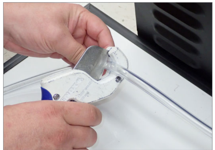
FIG. 3. Cut the drain line with tubing cutters.
