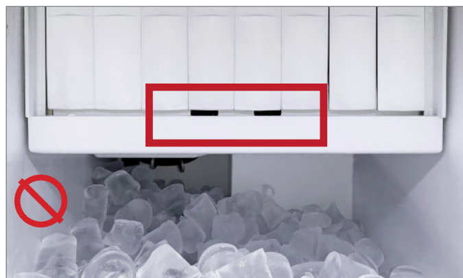
INCORRECT. Ice guide finger holes are visible.
