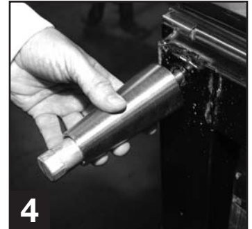
4 Thread leg into cabinet bottom frame rail.
