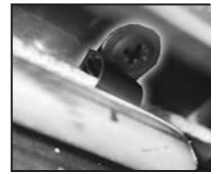
P-Clip keeps cord in-place (prevents cord damage).
