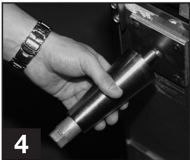
4 Thread leg into cabinet bottom frame rail.
