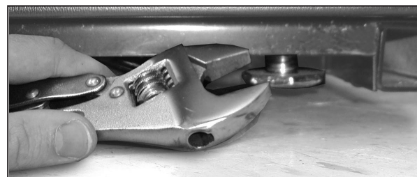
Use a crescent wrench to adjust leg levelers.
