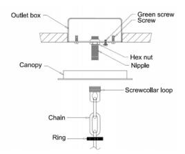
6. Fasten the ground wire to the green or bare copper wire in the outlet box or to the green screw on the crossbar.
