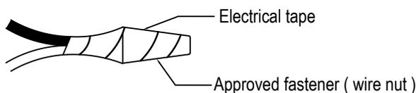
7. Connect the black fixture lead to the black wire in the outlet box. Fasten the joined wires as in step 6.
