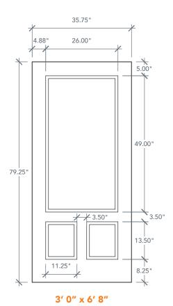
NOTE: BY REQUEST, DOOR HEIGHT COMES IN VARYING DIMENSIONS TO A MINIMUM OF 79". EXCESS WILL BE TAKEN FROM BOTTOM RAIL. ALL OTHER DIMENSIONS WILL REMAIN THE SAME.
