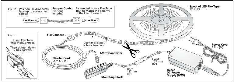
Tresco Lighting's LED Ultra Output FlexTape is to be mounted to a metal substrate for proper heat sinking. Failure to do so may lead to premature failure. To be used with Tresco DC Power Supplies Only. Indoor use only.
