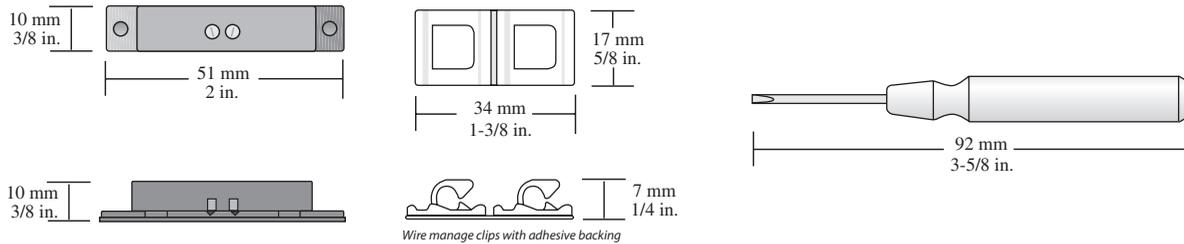
Wire manage clips with adhesive backing
