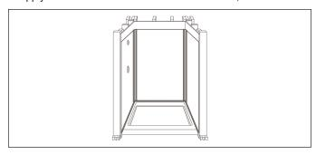
2. Apply 100% silicone sealant to the exterior edges, as shown. This silicone sealant is non-paintable.
