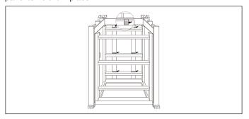
For corner shower wall installation use the following illustrated bracing design.
