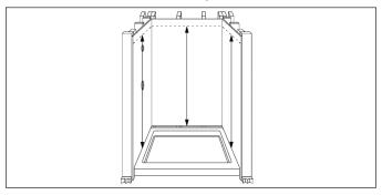
3. Transfer these measurements to both side panels and the back panel. Cut the bottom of the panels.
