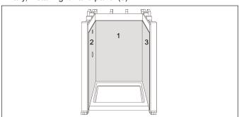
4. Firmly press the surface of each panel against the wall. It is important to apply hand pressure to the entire surface of the panel to bond it to the wall surface.
