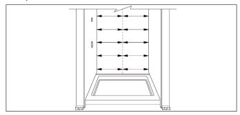
7. Transfer the measurements onto the front surface of the back panel.
