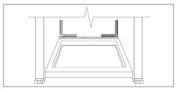
2. If the shower base is not perpendicular to the wall, use a level and draw a line around the alcove on all three walls. Measure the distance from the line to the top of the shower base.
