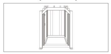
3. Install (wedge) three horizontal braces (six total) against the left and right wall braces.
