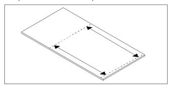
4. If the back panel must be cut (side-to-side) to fit the opening, find and mark the center of the back wall in the alcove opening. Use a level to draw a line from the shower base to a point above the height of the wall panel.
