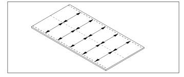
**Note:** The back panel can be cut **slightly** smaller than the opening because the side panels will cover any small gap (less than 1/4 inch).
