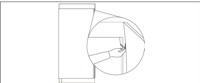
3. Place the panel, finished side facing up, on a flat surface. Place pieces of masking tape over the area where the saw contacts the panel.
