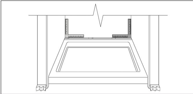
2. If the shower base is not perpendicular to the wall, use a level and draw a line around the alcove on all three walls. Measure the distance from the line to the top of the shower base.
