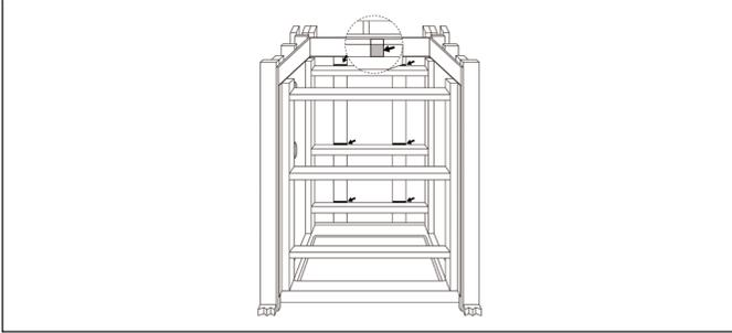
For corner shower wall installation use the following illustrated bracing design.
