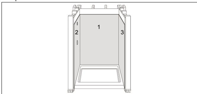
**Note:** For 60" wide shower, install first back panel, then seam trim or deco strips and second back panel. If not using seam trim, we commend placing 1/8 inch grout spacers between two back panels. (figure 5)
