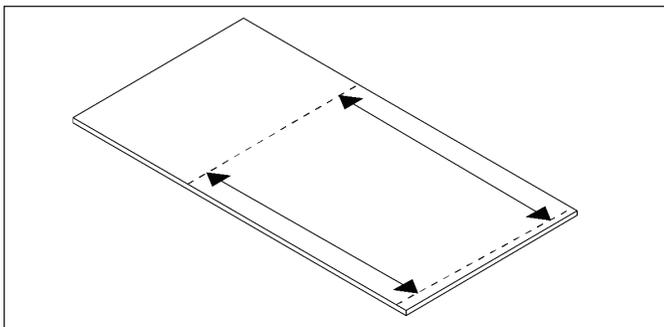
4. If the back panel must be cut (side-to-side) to fit the opening, find and mark the center of the back wall in the alcove opening. Use a level to draw a line from the shower base to a point above the height of the wall panel.
