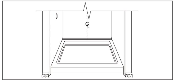
5. Place the panel, finished side facing up, on a flat surface. Using a pencil, lightly mark the center of the back panel.
