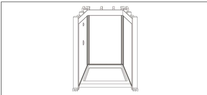
2. Apply 100% silicone sealant to the exterior edges, as shown. This silicone sealant is non-paintable.
