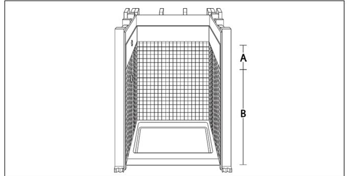
**Note:** Failure to use filler board to properly install the panels could result in water damage to floors, walls, or other portions of your building or home.
