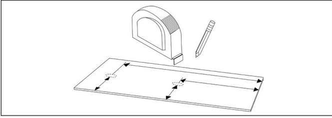
7. Cut clearance holes using a router, saber saw, or hole saw. Drill or cut from the finished side of the panel. For best results, when drilling, place a scrap of wood beneath the hole to ensure a clean cut.
