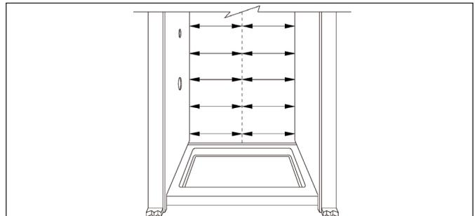
7. Transfer the measurements onto the front surface of the back panel.
