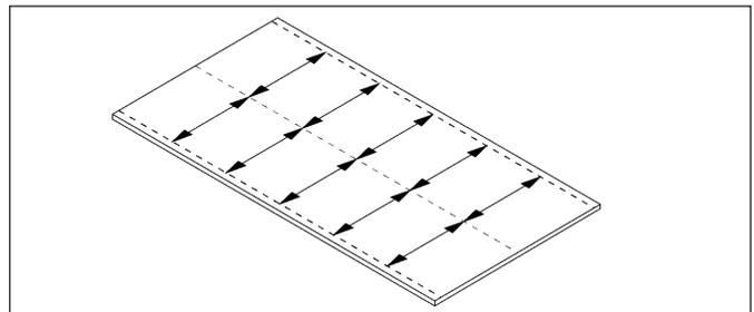
**Note:** The back panel can be cut **slightly** smaller than the opening because the side panels will cover any small gap (less than 1/4 inch).
