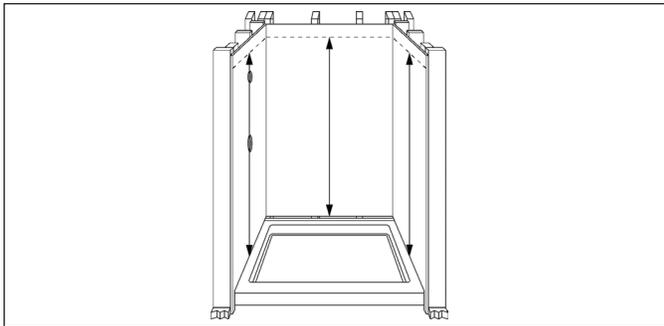
3. Transfer these measurements to both side panels and the back panel. Cut the bottom of the panels.
