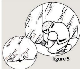
5. Firmly press the surface of each panel against the wall. It is important to apply hand pressure to the entire surface of the panel to bond it to the wall surface.
