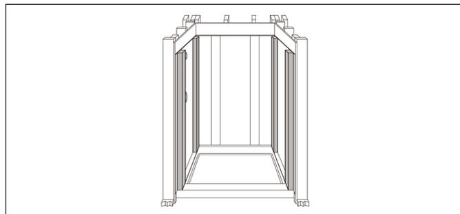
3. Install (wedge) three horizontal braces (six total) against the left and right wall braces.
