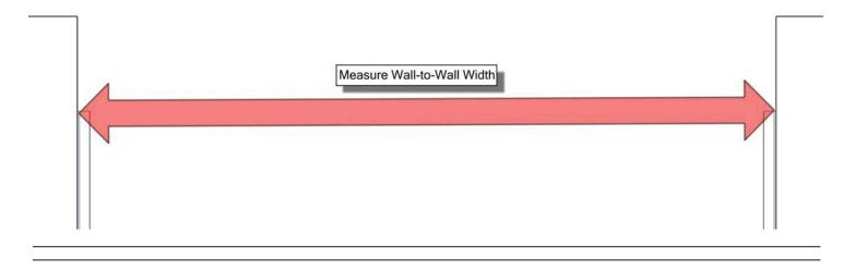
7 Subtract 1/2" from the measurement [T]. [T] - 1/2" = \_\_\_\_\_\_" [HC] Cut the Header to length [HC].
