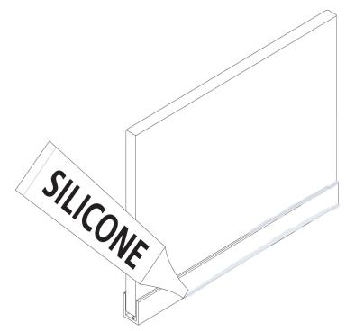
NOTE: DO NOT USE the shower until the silicone is completely cured. Check the tube of silicone for the manufacturer recommended cure time (typically 24 - 48 hours).
