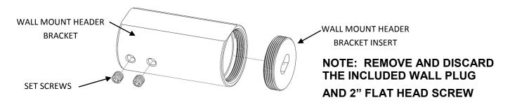
Next, screw the Header Bracket Insert onto the wall with the supplied #10 x 3" Flat Head screw. Install the Header Bracket Insert with the adjustment slot in the vertical direction. This will allow for a small amount of adjustment to make sure the header is level.
