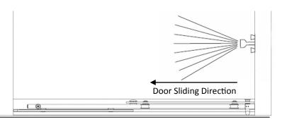
1 Determine location of the unit centerline on the threshold. From unit centerline mark location of panel centerline 1" towards outside of shower. Next, mark a continuous panel centerline on the wall the panel will mount to, starting where the threshold centerline meets the wall. Use a level to ensure the wall centerline is plumb and straight. The wall centerline should be a minimum of the unit height from the threshold.
