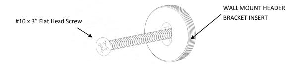
Reassemble the header assembly to the fixed panel glass and the wall mount header bracket. Check the header for level. Lightly tap the wall mount bracket to achieve level. Carefully remove the header assembly and completely tighten the Flat Head Screw from Step 9. Final install the header assembly to the panel glass and wall mount bracket. Tighten the set screws in the wall mount bracket.
