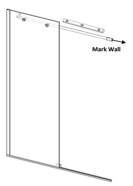
With the header assembly [8] mounted, use a pencil to mark the location where it sits flush against the door side wall as shown.
