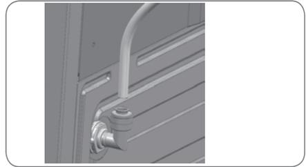
Step 3 ) Connect the PE soft tube.
