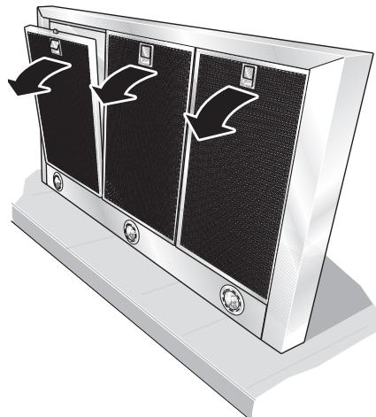
2. Remove the steel plate.
