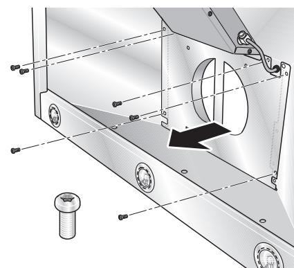
3. Remove the round duct plate.
