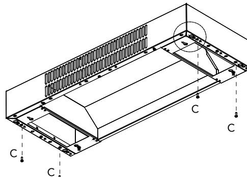
2. Install the deflector on top of the hood so that screws C go respectively into Side Slots on top of the hood and Side Slots on bottom of Deflector, slide the deflector frontward until stops.
