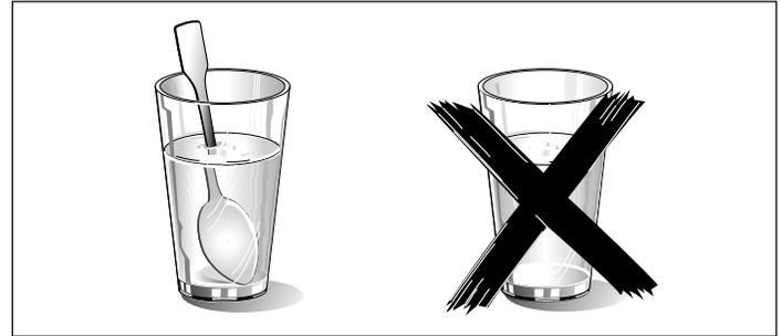
Liquids, such as water, coffee, or tea could be overheated. They can be heated beyond the boiling point without appearing to boil. For example, visible bubbling or boiling when the container is removed from the microwave oven is not always present. THIS COULD RESULT IN VERY HOT LIQUIDS SUDDENLY BOILING OVER WHEN THE CONTAINER IS DISTURBED OR A UTENSIL IS INSERTED INTO THE LIQUID.
