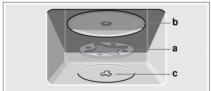
**Note:** Do not use the appliance if the turntable is not in place. Confirm that all parts are properly seated and that the turntable rotates freely when the microwave is operated.
