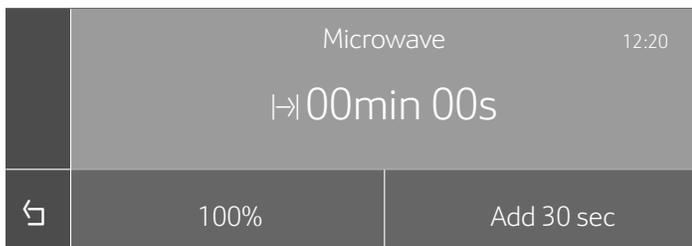
4. Touch the power level field and swipe to the left or right to select a different power level.
