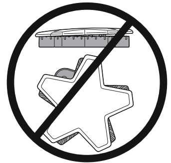
Incorrect burner cap
