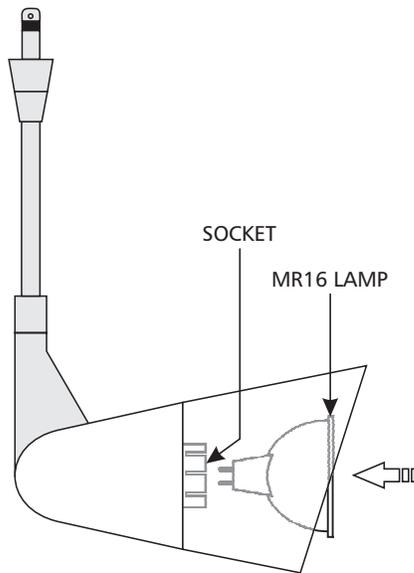
Use **MAX 50 Watt** type MR16 Front Cover Halogen Lamp.
