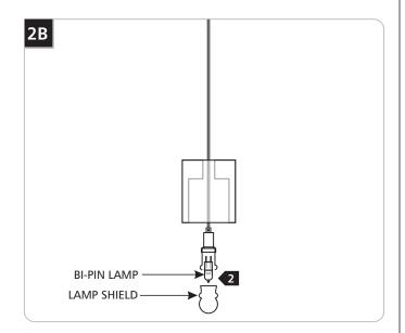
2 Remove the lamp shield and the old lamp.
