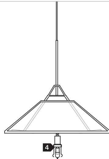
**3** Handle the new replacement lamp with a soft cloth to prevent the natural oils on the fingertips from collecting on the lamp. This will help extend the life of the lamp.
