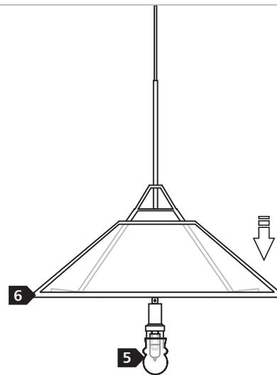
**5** Push the lamp shield onto the spring clip.
