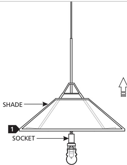
**1** Lift the shade up to expose the socket.
