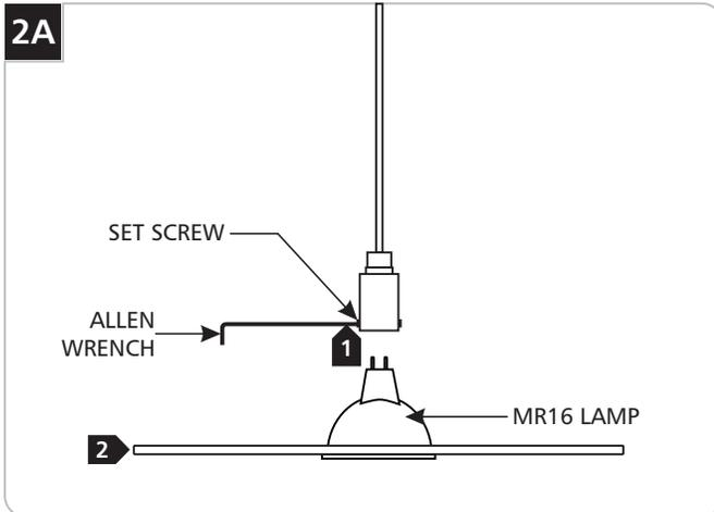
**1** Hold the glass with one hand and loosen the bottom two set screws with the Allen wrench.
