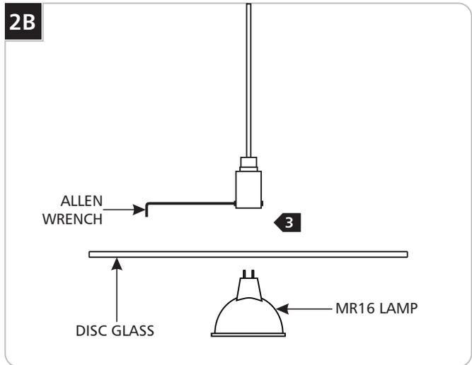
Use **MAX 50 Watt**, type MR16 Front Cover Halogen Lamp.
