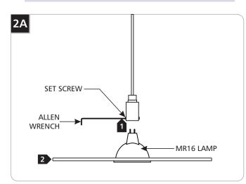
1 Hold the glass with one hand and loosen the bottom two set screws with the Allen wrench.
