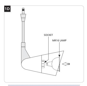
Use **MAX 50 Watt** type MR16 Front Cover Halogen Lamp.
