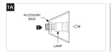
**CAUTION:** To reduce the risk of a burn or electric shock during relamping, disconnect the power to the fixture.
