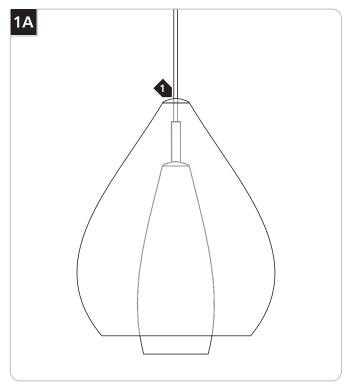
1 Feed the cord through the hole at the top of the outer shade.
