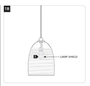
2 Push the lamp shield onto the spring clip.
