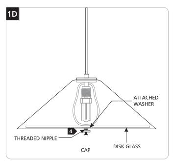
A Replace the disk glass and fasten the cap to the threaded nipple tight to secure the disk glass properly in place.
