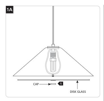
1 Loosen the cap and carefully remove the disk glass to expose the socket.
