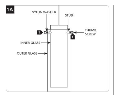
1 Line up the outer glass holes with the inner glass studs and secure the outer glass to inner glass with provided thumb screws and nylon washers.
