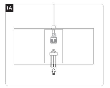
Use **MAX 32 Watt** GX24Q-3 base triple tube compact fluorescent lamp.
