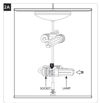
Use MAX 32 Watt GX24Q-3 Base Triple Tube Compact Fluorescent Lamp with each socket.
